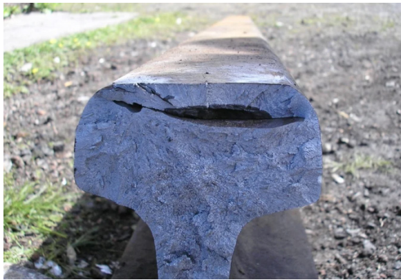
Figure 1 - Quenching cracks in the hardened layer at the end of the rail
